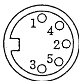
Figure 4.6 Layout of DC CONTROL Connector Pins (as viewed from chassis rear)
